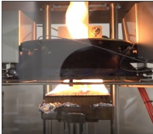
Figure 2. Timber surface radiated to get burned
